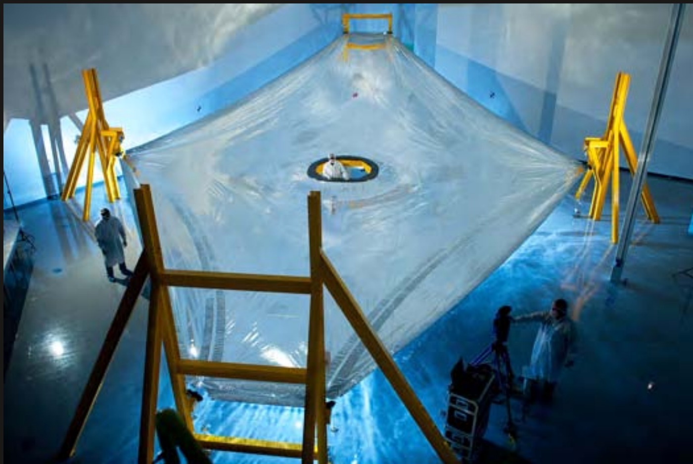
Technicians at ManTech International's facility in Huntsville, Alabama, check the layer 3 sunshield test membrane mounted on a fully simulated flight structure. Each of the five tennis court-sized sunshield test layers will be 3D shape-tested to validate computer models. Photo credit: Northrop Grumman.
