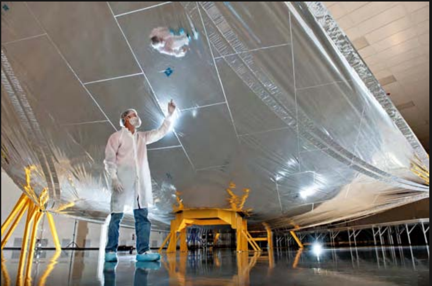
Technician checks layer 3 sunshield test membrane mounted on a fully simulated flight structure at ManTech International's facility in Huntsville, Alabama. Credit: Northrop Grumman.
