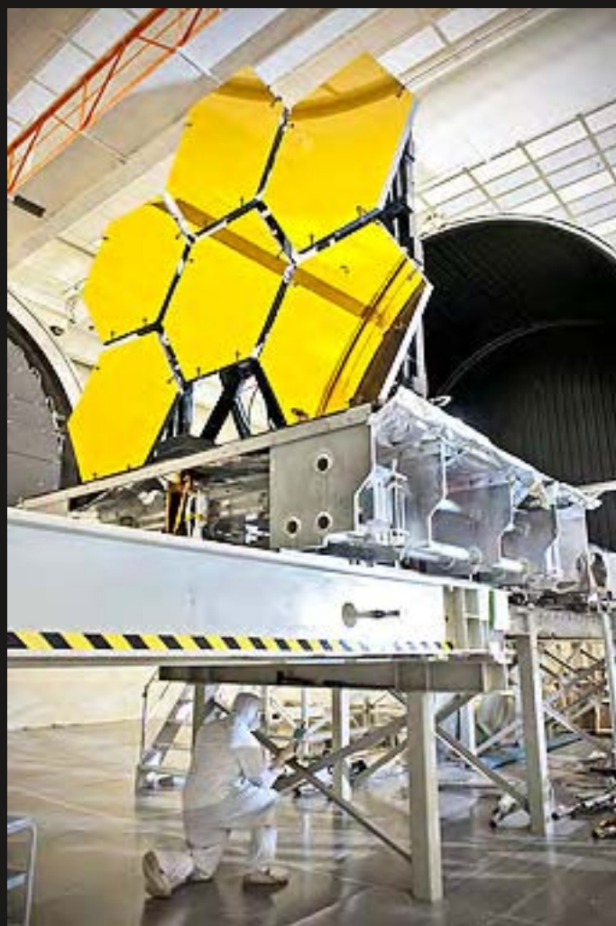
Primary mirror segments outside a chamber in the X-ray and Cryogenic Facility at NASA's Marshall Space Flight Center, Huntsville, Alabama. All primary segments are chilled to near minus 400 degrees Fahrenheit to insure they perform as expected in the deep cold of space. Credit: MSFC/NASA
